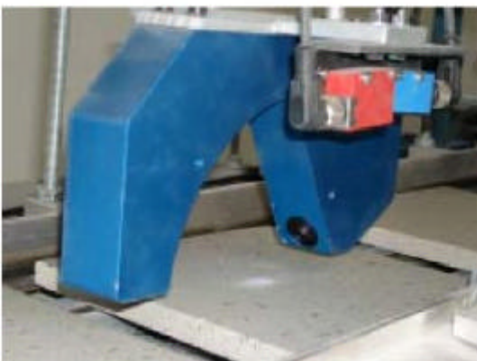
Gloss degree monitoring at plates of stone
