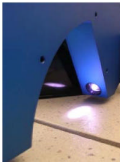
Online gloss measurement at ceramic parts
