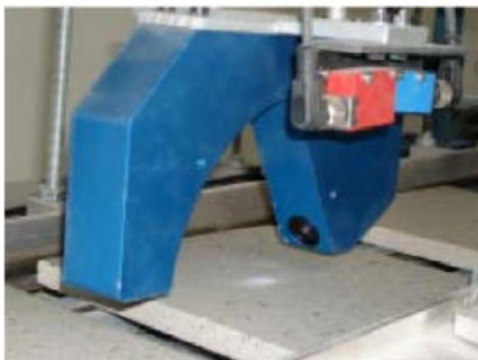
Gloss degree monitoring at plates of stone
